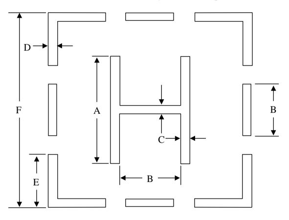
$\begin{array}{c} \underline{DIMENSIONS} \\ A = 0.6 \ F \ (MAXIMUM \ OF \ 20M) \\ B = 0.5 \ A \end{array}$
